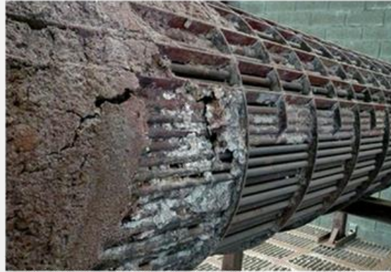
AFTER THERMAL CLEANING
